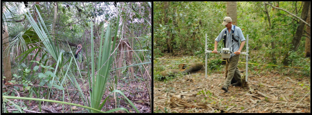
FIGURE 2. Zeroing the susceptibility meter between readings under typical ground-cover conditions (left); conducting magnetometer survey in a cleared location (right).
